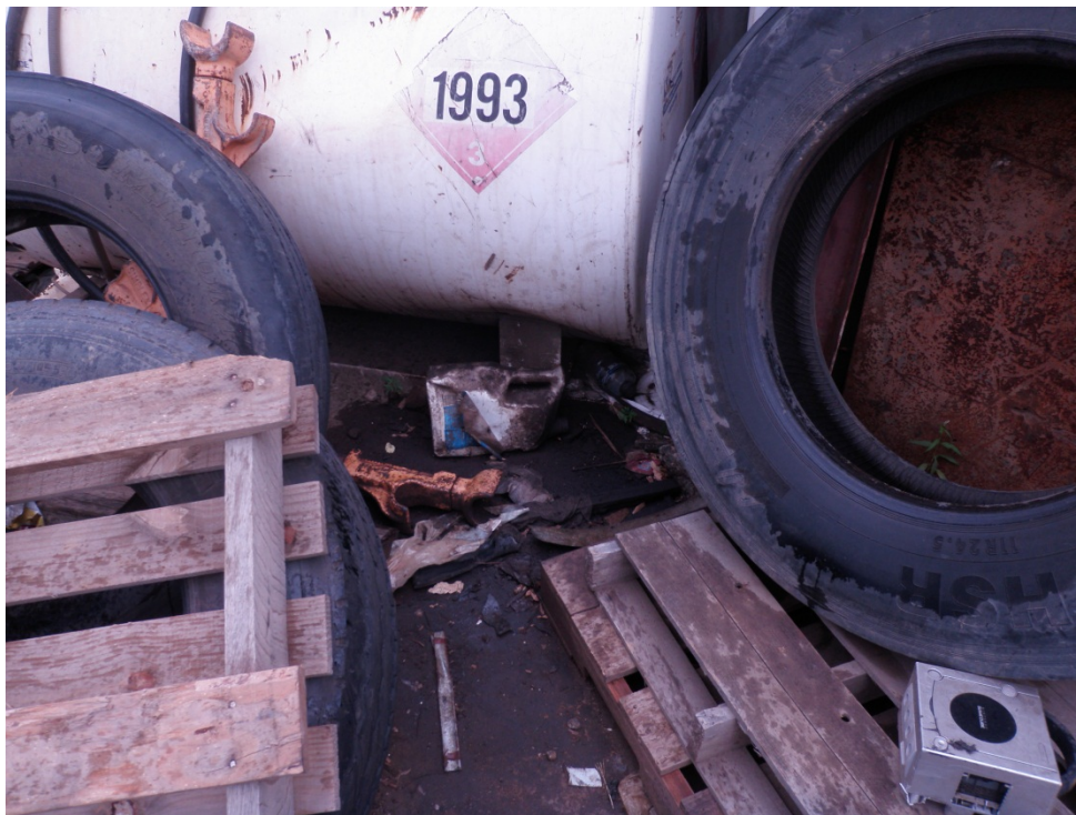
Photo #6: Staining around AST in northern portion of Square 0605, Lot 0802
