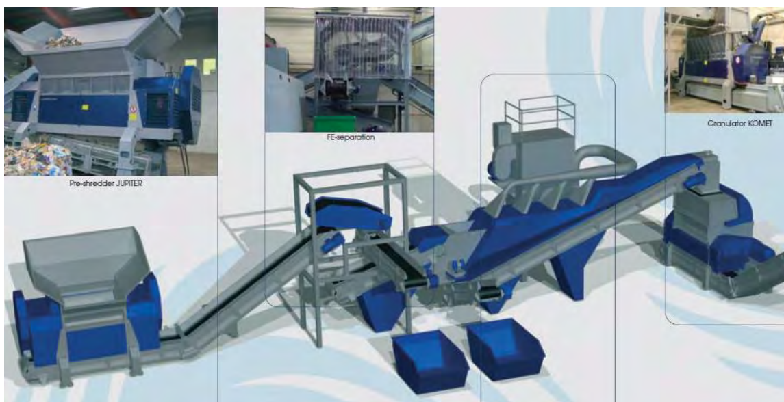
VDRS Process Engineered Fuel (PEF) Equipment Design (similar to RDF)
