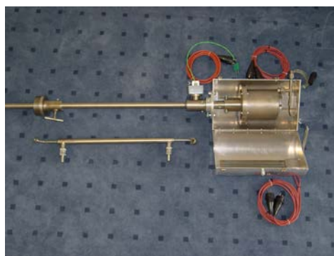
High-dust-probe with opened filter box
